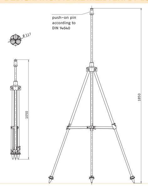
max. extension height 1.85 m inserted length 1.05 m Weight 5.8 kg max. centred load 18.00 kg Mounting bolts according to DIN 14 640 External tubes fire red, powder-coated Telescope tubes zinc-yellow, anodized, all tubes can be locked with secure stops at any height, for uneven, difficult terrain, all tripod legs can be extended individually For use with 2 floodlights, we recommend our 3 supporting bridges and our DUO-LIGHT. captive belt with lock to secure the 3 legs Transport safety
